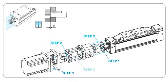
Tighten the screws on the coupling halves in the coupling tightening torque.
