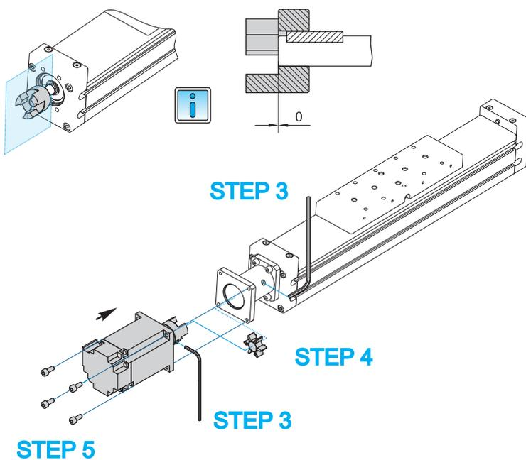
**STEP 3:** Ensure that the coupling halves and the drive journals are correctly aligned.
