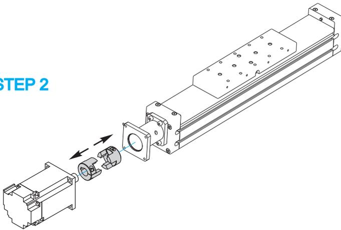
**STEP 2:** Place the coupling halves on the drive journal of the Linear Unit and the motor.
