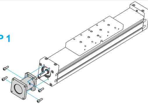
**STEP 1:** Attach the motor adapter on a pre-prepared location on the Linear Unit and screw down.
