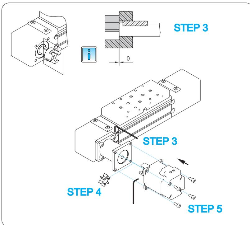
**STEP 4:** Insert the coupling spider into one of the coupling halves.
