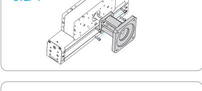
**STEP 2:** Place the coupling halves on the drive journal of the Linear Unit and the motor.
